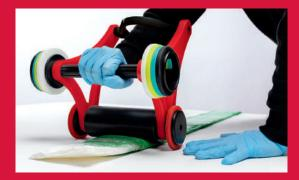
It's a great option for small laterals and connections and can be used inside buildings and small spaces due to the compact design, providing there is a flat surface to impregnate the liner.
